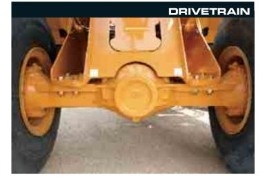
The 621E wheel loaders use a torque sensing autoshift transmission with four forward gears and three reverse ratios. Top forward speed is 38.6 km/h.
