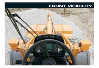
Case E Series wheeled loaders benefit from a greatly enlarged operator's cab, with up to 15 % more floor area. The tapered design is longer and wider than the D Series, offering more internal space for the driver and reduced noise levels that are among the quietest in the industry.
