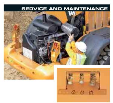
Thanks to the mid-mounted cooling module design, the engine sits at the rear of the machine, where it contributes to the counterweight. A single-piece electrically-operated engine cover. lifts clear of the engine for service and maintenance, and all daily checks can be easily reached from ground level, with fluid sight gauges on all reservoirs.
